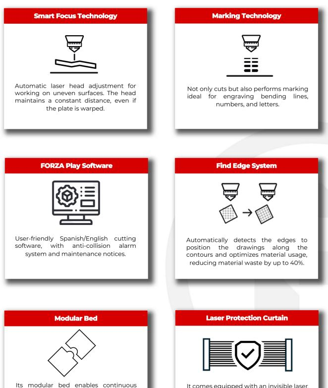
It comes equipped with an invisible laser safety curtain installed along the entire movement range of the cutting head. If an obstacle enters the work area, the system immediately stops the machine to prevent a collision.
