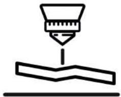
Automatic head for working on uneven surfaces, no matter if the plate is warped, the head will maintain a constant distance throughout the cut.
